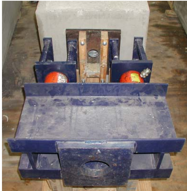
Figure 3-11 Specimen Ready for Installation of Tendon
