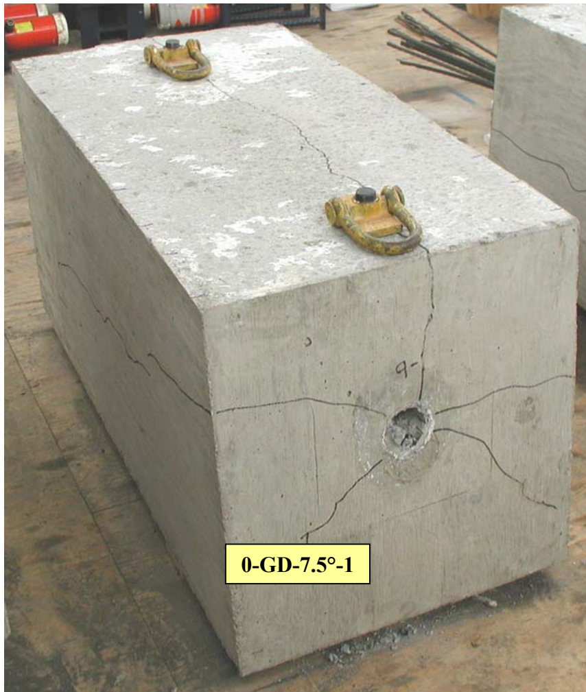
Figure 4-39 Profile of Specimen 0-GD-7.5°-1 after Testing
