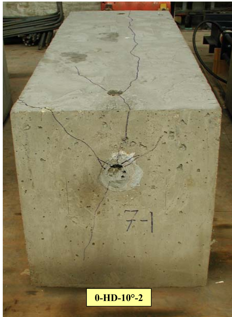
Figure 4-63 Photo of Specimen 0-HD-10°-2 after Testing
