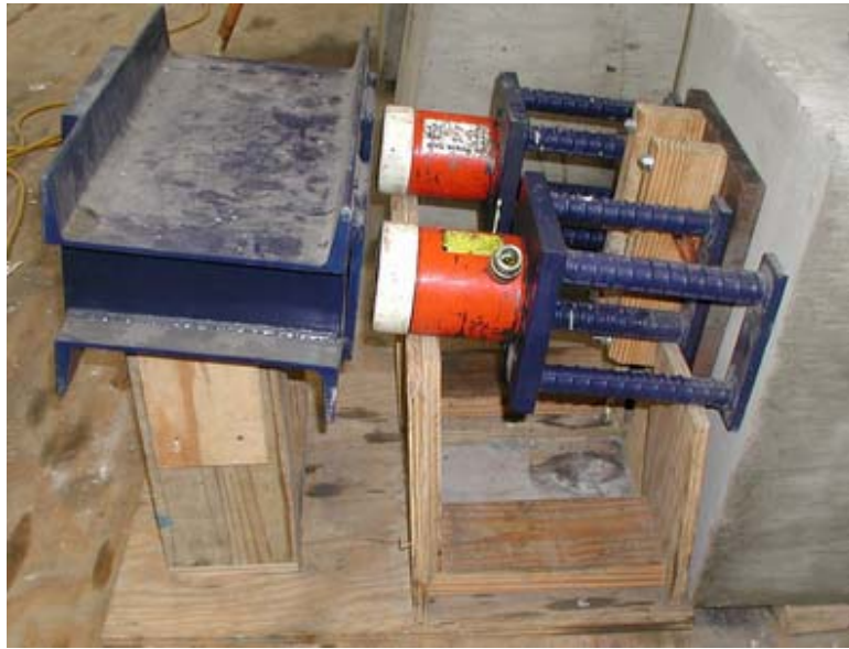
Figure 3-10 Prestressing Equipment on Supports
