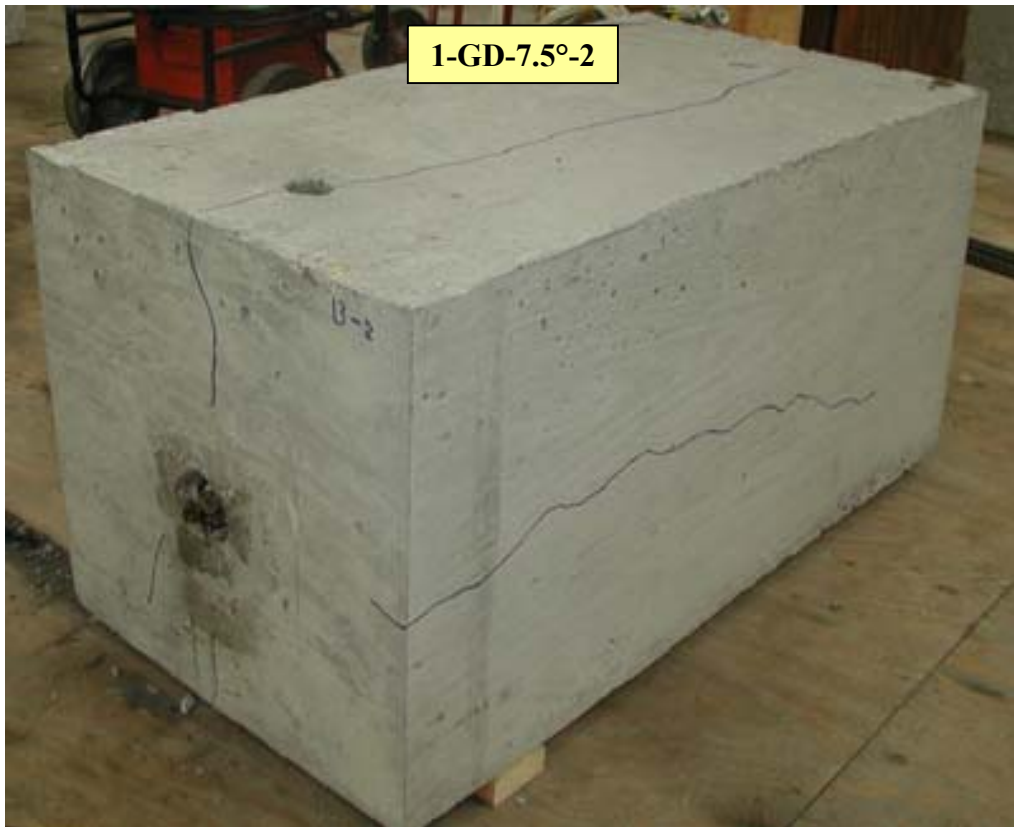
Figure 4-54 Photo of Specimen 1-GD-7.5°-2 after Testing
