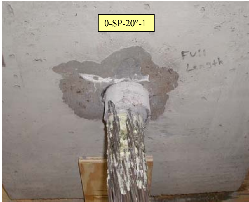
Figure 4-7 Live End of Specimen 0-SP-20°-1 after Testing
