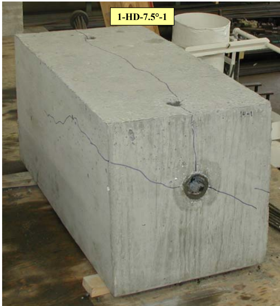
Figure 4-79 Photo of Specimen 1-HD-7.5°-1 after Testing
